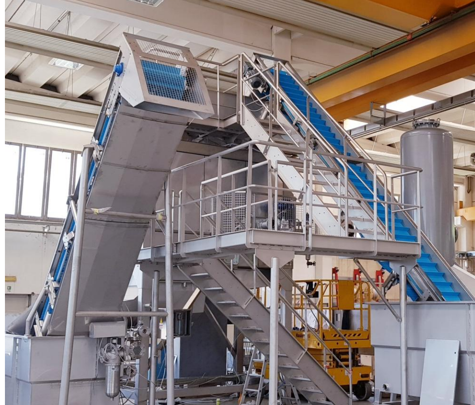
LADDERS FOR INSPECTION AND WASHING FOR THE LOADING AND DISCHARGING ELEVATORS
