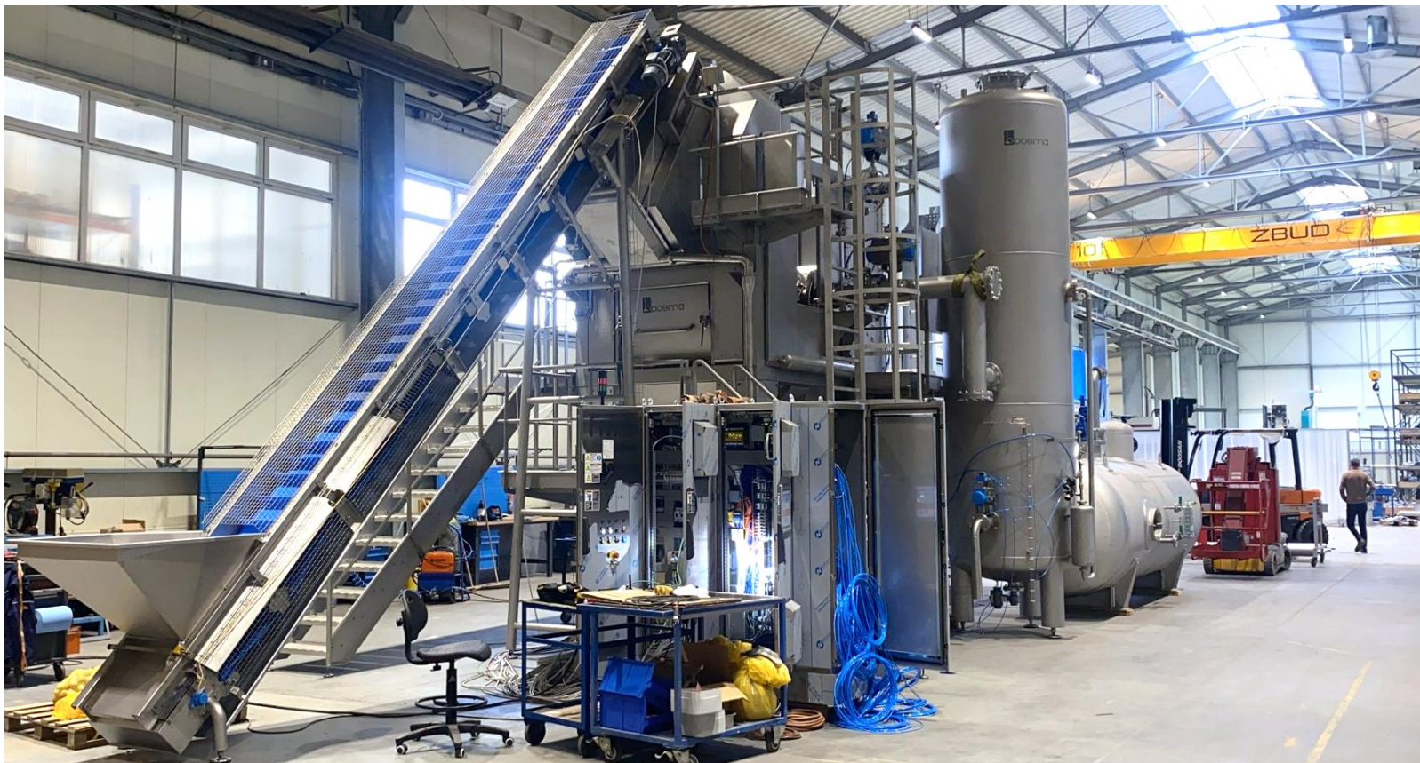
BLUE BELT FOR LOADING ELEVATOR AND BATCHER FOR PRODUCT FEEDING TO THE PEELER, SOLUTION FOR FRUIT PROCESSING
